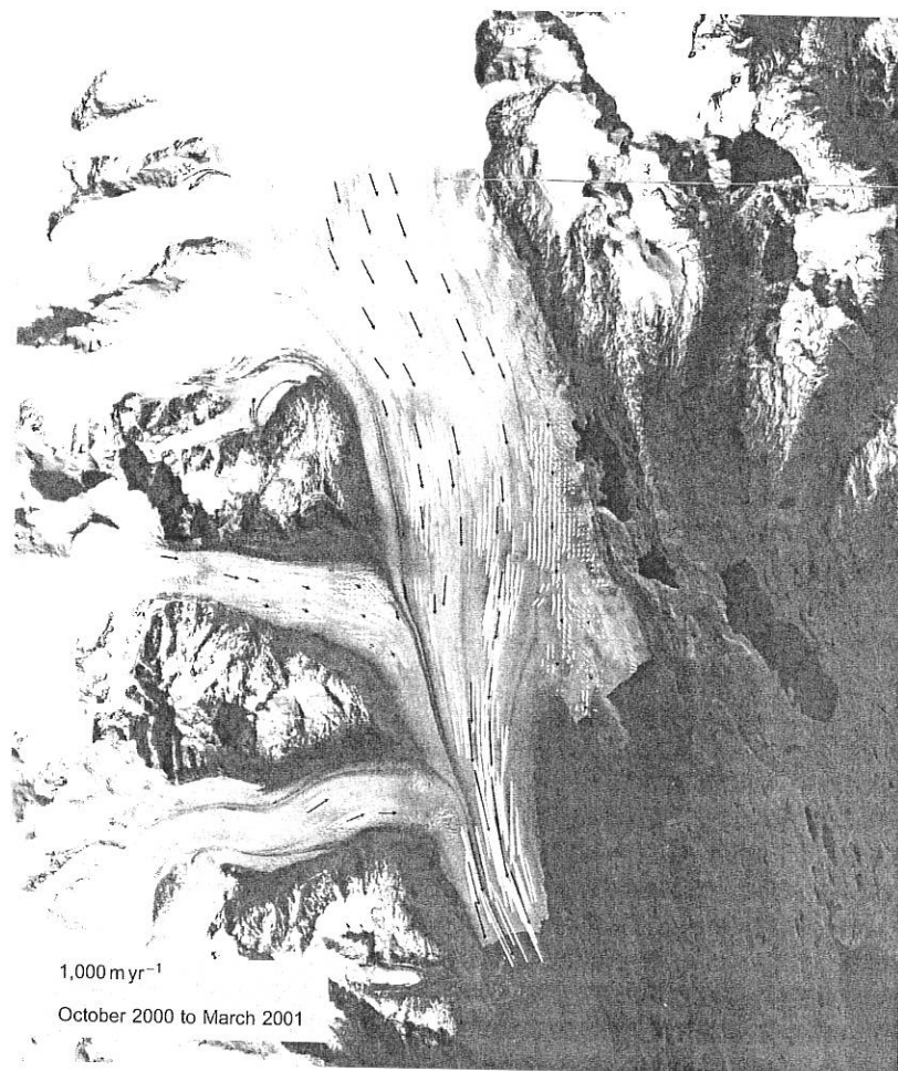
Figure 5.7. Landsat ETM+ image acquired 14 October 2001 showing Upsala Glacier, South Patagonia. All velocity vectors obtained from cross correlation-based feature tracking between October 2000 to March 2001 are overlaid as white line segments, and a subset of these are overlaid as black arrows for clarity. Ice surface speed ranges up to just under 2,000 \text{ m yr}^{-1} . The fast-moving calving front is approximately 2 km wide.
