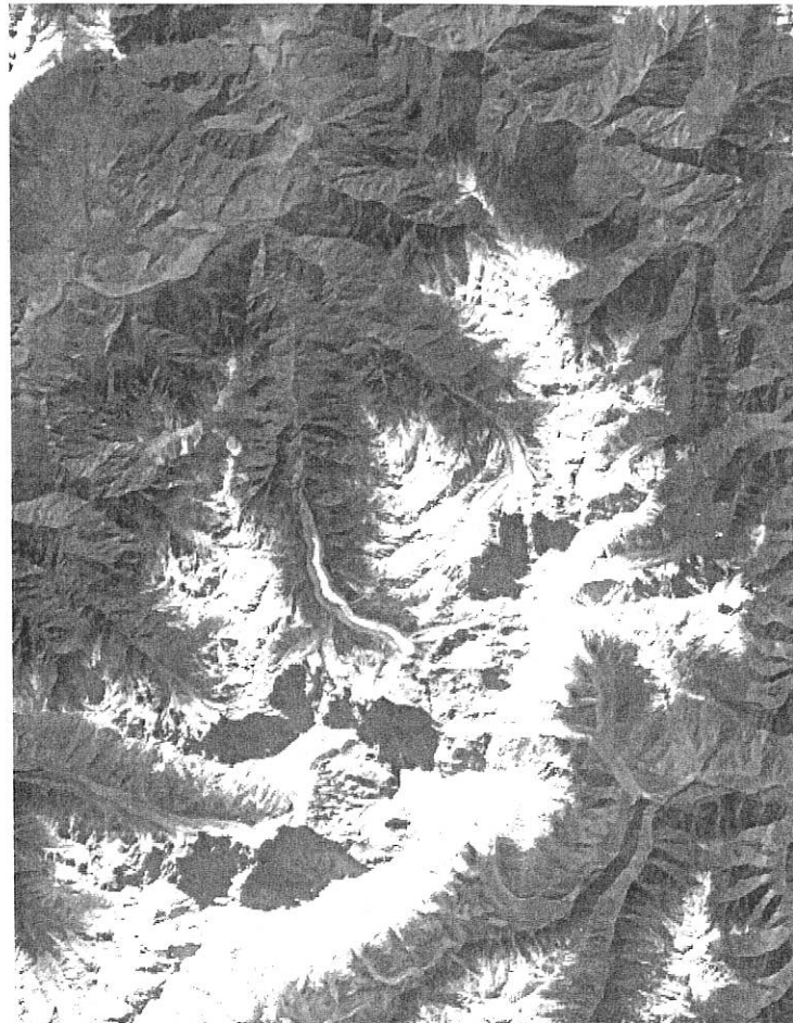
Figure 5.1. SPOT 2 HRV panchromatic image of Nanga Parbat in northern Pakistan. Image acquisition date is 31 October 1991 at 06:05:08 UMT, with \theta_s and \phi_s values of 50.2^\circ and 167.5^\circ , respectively. Direct irradiance variations (cast shadows) make it difficult to use the imagery for mapping or biophysical applications. Image width is approximately 40 km and north is toward the top of the page.
