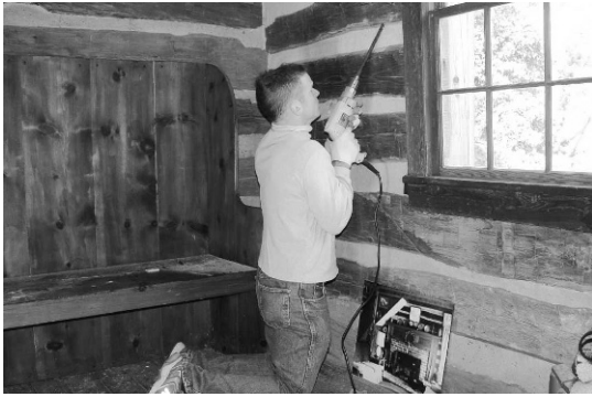
Figure 2. Extracting a core from the rounded portion of a log in the interior of the Hoskins House with a hollow tubular drill bit attached to a 0.5 inch (1.3 cm) variable speed drill.
